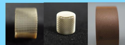
**Figure 8:** Thin films of TiC deposited via E-beam deposition on dielectric resonators. The fishnet pattern of the films ( $300\mu\text{m} \times 300\mu\text{m}$  squares) helps the dielectrics to retain their high Q (4x higher than continuous film) while offering a source of free-electrons.
