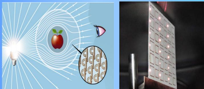
**Figure 1:** An illustration of an invisibility cloak (left)[8]. On the right an array of ring resonators of two different sizes with gaps of  $\sim 160\mu\text{m}$  are shown. The resonators are subject to radiation from a patch antenna at 2.41GHz. The result, as seen above, is plasma generation in the large rings' gaps [4].
