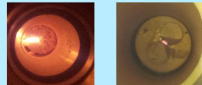
**Figure 7:** Plasma generation in atmosphere is visible in dielectrics subject to 1000W of multimode microwaves at 2.45GHz. On the left is a  $\text{Zr}_{0.8}\text{Sn}_{0.2}\text{TiO}_4$  resonator and on the right are two identical  $\text{CaTiO}_3$  resonators designed to resonate in TE011 and HEM12 $\delta$  modes respectively when excited by 2.45GHz microwaves. Thanks to Jipeng Cheng and Dinesh Agrawal for assisting with the plasma experiments.
