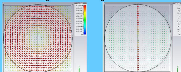
**Figure 5:** Simulations showing electric-field distributions of TE011 mode in a dielectric resonator (left) and the field distribution of the same mode in a split resonator. Note: Scales for electric fields are different for each image.
