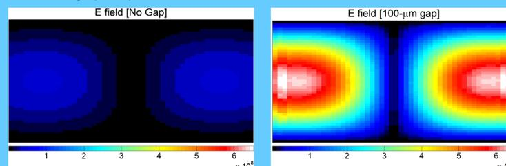
**Figure 6:** Simulations showing electric-field magnitude (V/m) in a split (right) and non-split dielectric resonator. These cross sections correspond to the center of the resonator parallel to the split.
