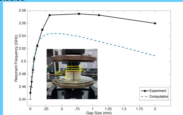
**Figure 3:** Resonant frequency of the TE011 mode is shown as a function of the gap distance between the two halves of the resonator. In the inset, a Haki-Coleman setup for studying dielectric properties is shown with the ZST resonator.
