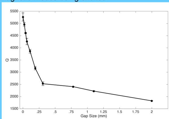
**Figure 4:** Quality factor of the resonator versus the gap distance.
